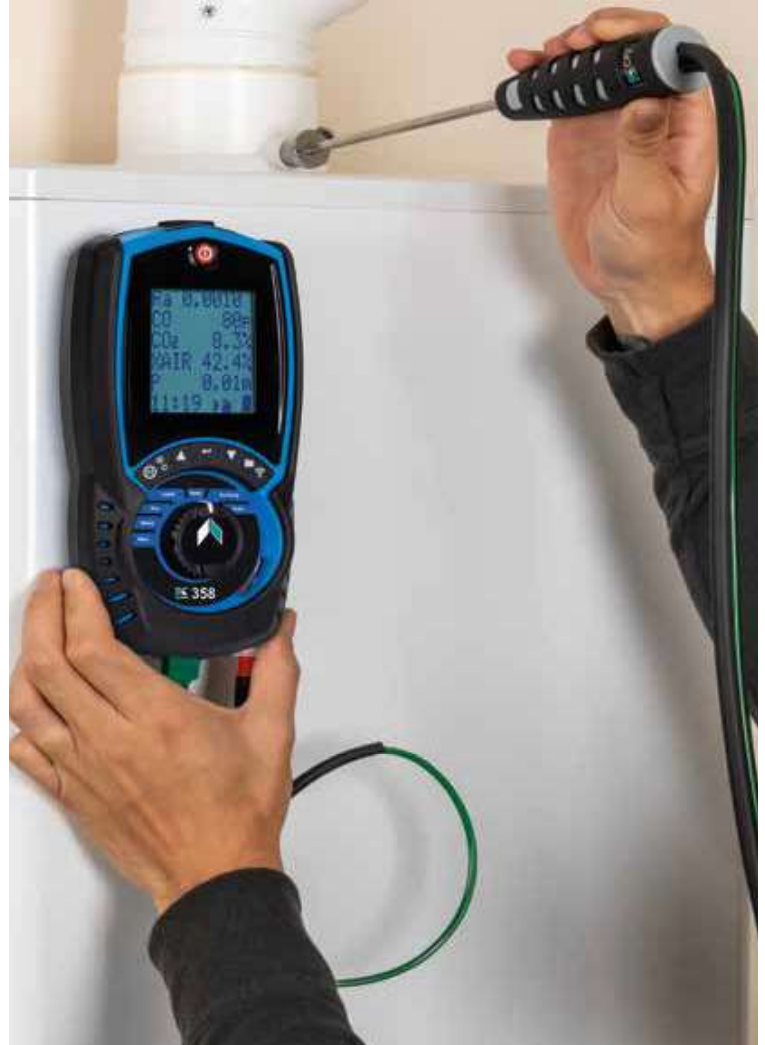
Flue Gas Analysis
